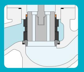
In this type, the trim characteristic is achieved through the profile of the port opening of the cage. Multiple ports enable streamlined flow. Large cage guiding, interchangeability of trim parts and high flow capacity are the defining features of this design.
