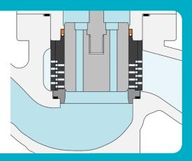
For this purpose flow under is preferred for gas application. Flow over may lead to generation of low frequency secondary noise due to pressure drop at the seat due to increased volume flow of the expanded gas.
