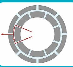
In gas applications, multiple cage designs are used to reduce the noise and vibration caused by abrupt pressure reduction in high pressure drop. The fluid flow is split into numerous small flow streams. There by substantially shifting the frequency of the generated noise beyond the audible spectrum. The pressure is dropped in many stages in velocity controlled manner though an expanding flow passage.
