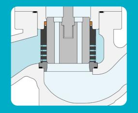
Single and multiple heavy section 'drilled hole' cage design offers low pressure recovery that reduce the potential for excessive noise, cavitation, vibration and erosion. The CC trim range has been designed to operate on all fluid combinations, both clean and dirty service. The CC range of trims is normally the first choice for medium to relatively high pressure drop applications.
