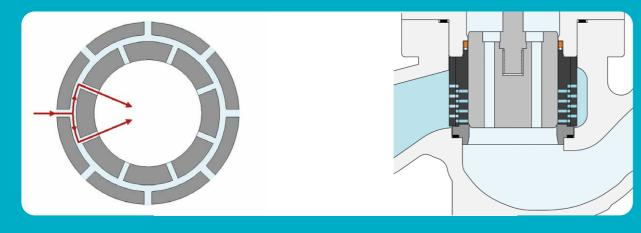
The erosive effect of cavitation is controlled by reducing the kinetic energy of the fluid by splitting the flow into many small flow streams. Multiple stage pressure let-down offered by 2CC trims results in low pressure recovery, thereby reducing the possibility of cavitation. The internal flow resistance offered by co-mingling of the adjacent flow streams acts as additional pressure drop stage, further reducing the pressure recovery.
