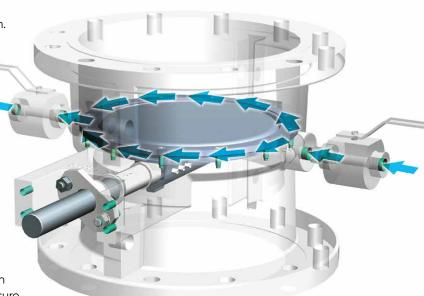
Typical sealant flow path
