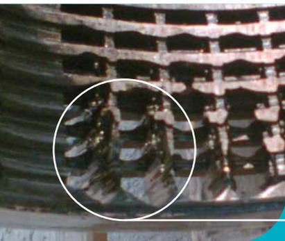
Previously, OEM control valves were failing in as little as 44 days.
