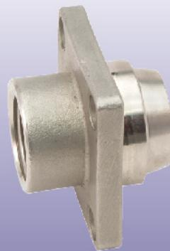
The conventional end cap and seat retainer was one piece design that made the end caps extended into valve body, creates a problem when repair and maintenance required, it is very difficult to remove end caps from valve body when valves mounted on pipeline, especially when ball valves was welded on pipeline.
