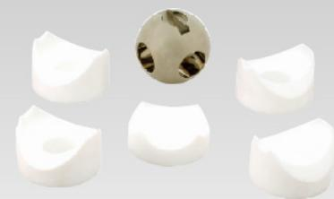
The cavity filled seats are designed to fill the dead space between the ball and valve body, minimize problems with trapped fluid in the valve body that can contaminate the process. Mars Cavity Filler Seats fill 95% of the dead space between valve body and ball, while others' cavity filled seats of 3/4/5-way ball valves can only fill maximum 80% of the dead space
