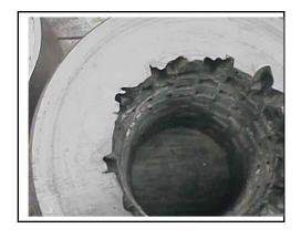
Severn's experience of severe service applications and investigations into the failure modes of many OEM's trims has shown that the use of vertical turns and separator plates in more erosive applications often results in premature failure of the trim.
