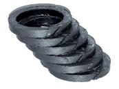
**Graphite packing:** These are self lubricating and does not require external lubrication. Relatively they offer higher friction and are suitable for a wide range of temperatures from -196°C to 450°C.
